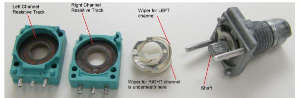
Above is the pot broken apart. Note there are two separate channels (one for left, one for right). **Also very interesting**: note that *each* channel has *TWO* wipers for redundancy (it's a little hard to see in the picture, as I've accidentally bent the two wipers so they are touching each other). This helps reduce any crackle or dropout when moving the pot, since at any time, at least one of the wipers *should* be in contact with the resistive track.
