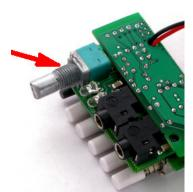
Pictured above is a typical 9mm pot, shown in its natural habitat inside the XM5 headphone amp. The 9mm refers to the pot's body size. It is a mechanical "**dual-ganged**" pot, consisting of two isolated sets of wipers, which scrape against two isolated sets of tracks of resistive material. "Dual-gang" means the pot consists of two separate potentiometers (one for the left audio channel, one for right) which share the same shaft
